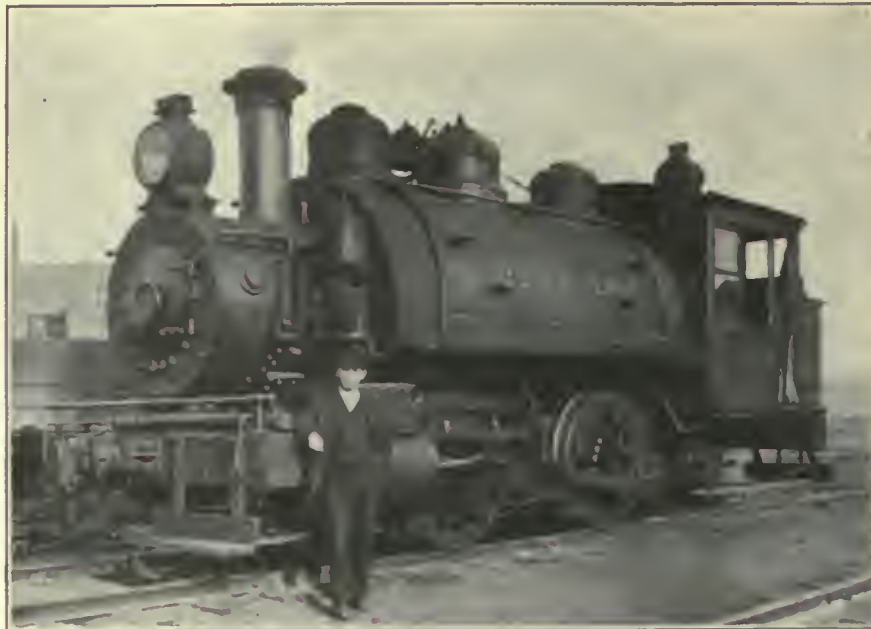
FIG. 389. LOCOMOTIVES. Switching Locomotive of the Four-wheel Type. At present, only a few locomotives of this type remain in service in Chicago. Illinois Northern Railway.
